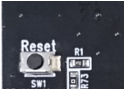
SW1 Reset button, low active
